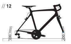
Place fork on front hub with correct lower axle adapters. Tighten your front axle.
