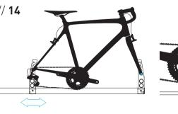
Adjust position of rear hub according to your wheel base. Place rear drop-outs on rear hub with correct upper axle adapter. Thighten your rear axel. Always choose lowest possible level at rear hub according to chain wheel size.
